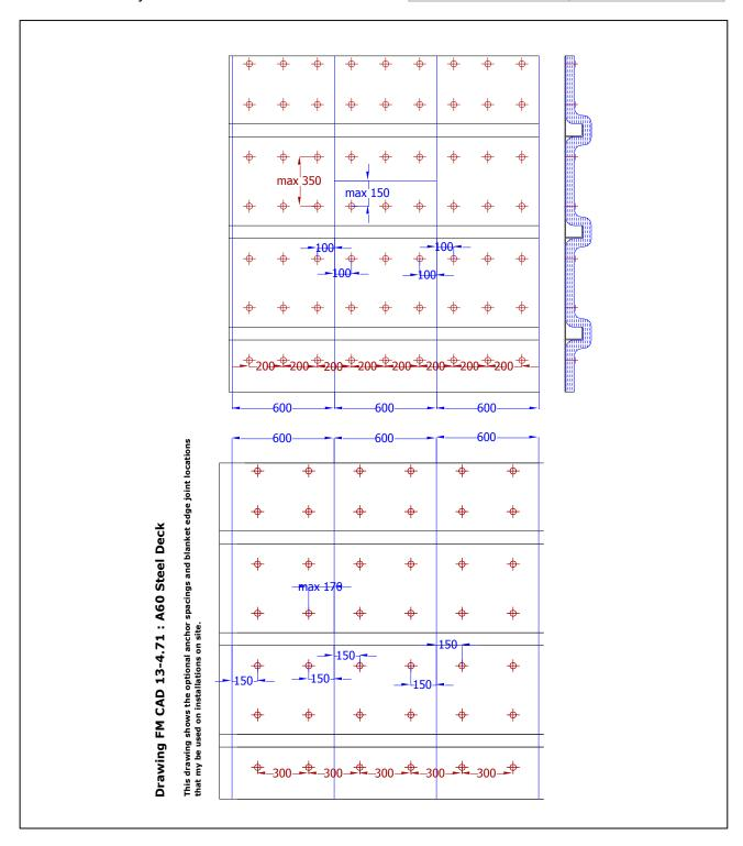
Blanket may be compressed from 65mm up to 45mm (i.e. 30%) thickness. Pin length to be from 50mm to 80mm typically.
