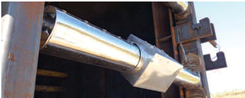
RES system after second explosion test.
