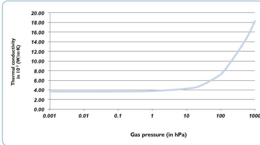
Thermal Conductivity (Panel Core) DIN 52612
