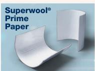
Superwool Prime Paper is manufactured using Morgan's newest fibre chemistry with a classification temperature of 1300°C (2372°F). Using patented low-shot technology fibres in a non-woven matrix with special organic binders, it has high strength for various applications.
