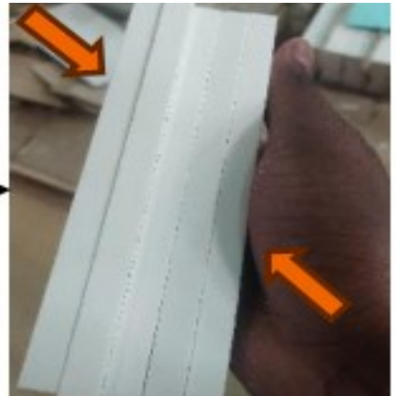
Figure 1 Bubble alumina embedded between high alumina tile – Sticking after firing
