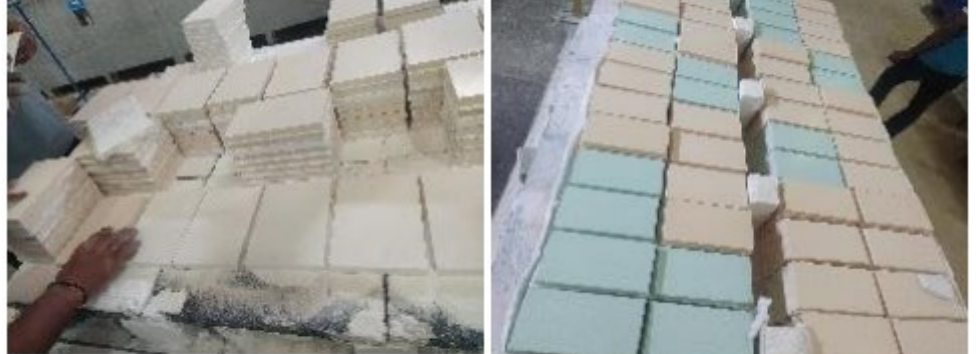
Figure 4 & 5: Separator sheets in production process
