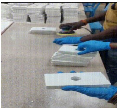
Figure 2 Tapping and Buffing to separate and clean the tiles
